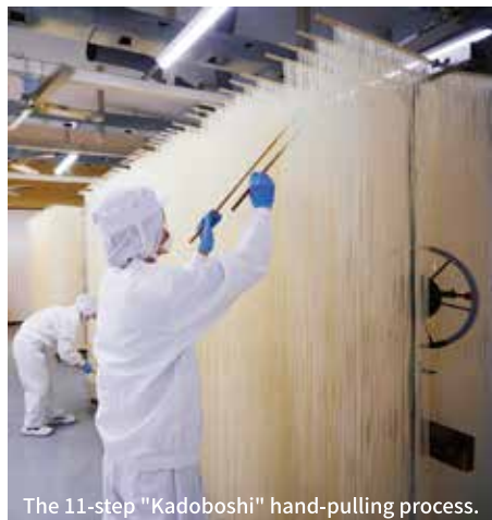
The 11-step "Kadoboshi" hand-pulling process.
